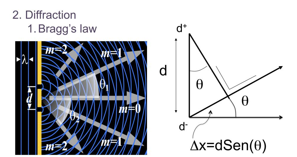
Wave from d<sup>+</sup> is  $E=E_0e^{i(k^*x+\varpi t)}$ Wave from d<sup>-</sup> is  $E=E_0e^{i(k^*(x+\Delta x)+\varpi t)}$ On phase: k\* $\Delta x=m2\pi$  (m=0,1,2,..) 2. Diffraction1. Bragg's law
